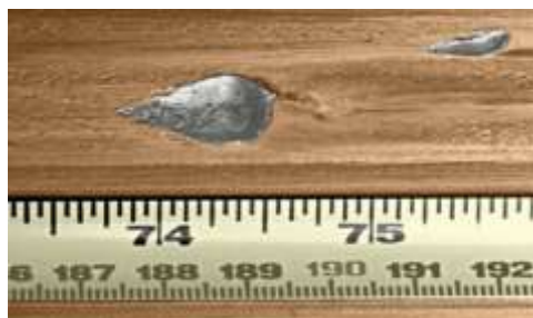
Figure 2 : Typical gouge on copper rail [McNab et al., 2011]
